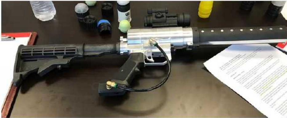
(Left) Working Prototype of Compressed Air Fired Launcher
