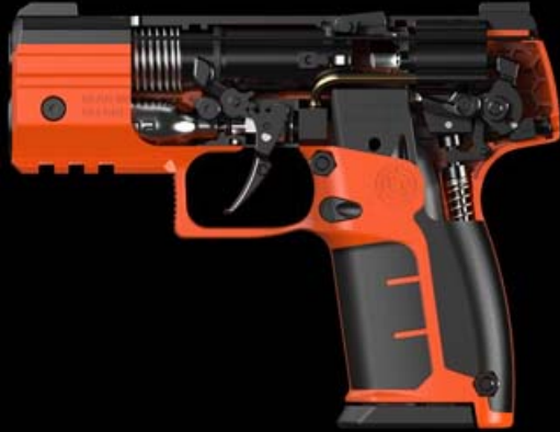
Byrna SD – Internals Cutaway
